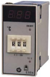
ESEN Coding setting, number indication thermoregulator Outer dimension: 48x96x110mm Hole dimension: 45x92mm
